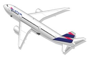
Boeing 787-8 - Dreamliner Capacity: 247 passengers Length: 56.72mts / 186ft Wingspan: 60.13mts / 197ft Maximum takeoff weight: 227.930kg / 251ton Emergency exit: 8 Toilet facilities: 6
