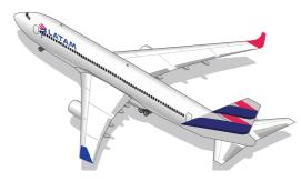
Boeing 767-300 Capacity: 221-238 passengers Length: 54.2mts / 177ft Wingspan: 47.16mts / 155ft Maximum takeoff weight: 184611kg / 203ton Emergency exit: 8 Toilet facilities: 6-7
