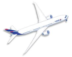
Boeing 777 **Capacity:** 410 passengers **Length:** 73.08mts / 214ft **Wingspan:** 64.80mts / 209ft **Maximum takeoff weight:** 346,544kg / 382ton **Emergency exit:** 10 **Toilet facilities:** 10
